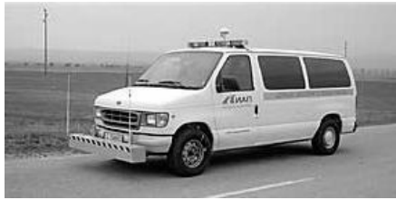
Fig. 3. Dynatest road surface profilometer, model 5051 MK II L3.2cg, used in Bulgaria [3].
