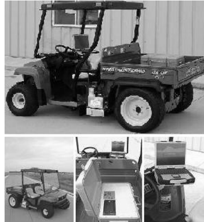
Fig. 6. Lightweight profiler, Ames Engineering, model 6200 Lisa, class I (ASTM E950-98) [3].
