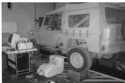
Fig. 16. Measuring system in the four-post laboratory.
